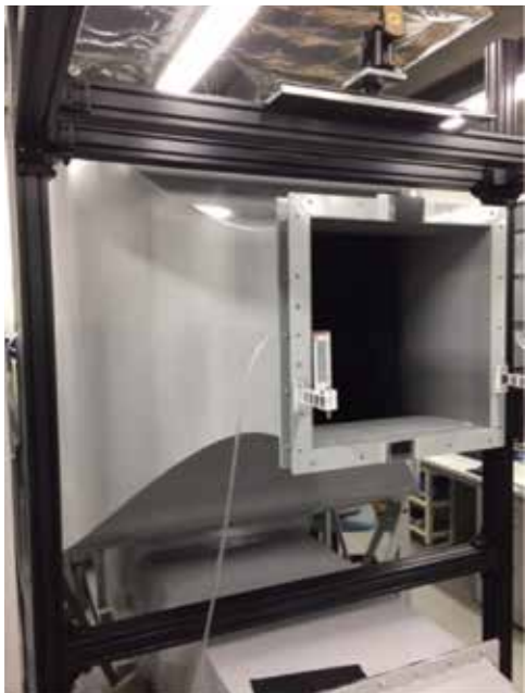
Wind tunnel equipment with 400 × 400 mm outlet
