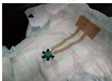
5 cells in series (0.34 mW)
